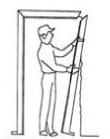
Slip strike jamb over wall.Insert tongues on head into slots at the top of the strike jamb.
