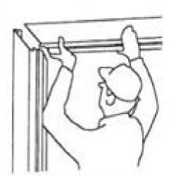
Slip head over wall-inserting tongues on head into slots at the top of the hinge jamb.
