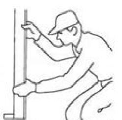
Slip hinge jamb over wall,into position.
