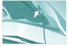
Secure the strut in one of the two notches, according to the height required, to hold the bonnet open.
