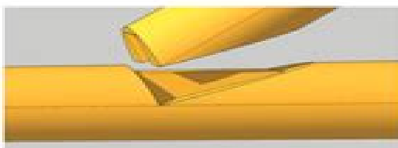
Figure 25: The hinge point is half way through the log. If we removed all that wood from the tie beam, it would be much too weak. So we leave a large block of wood — a tenon—in the beam.
