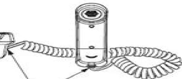
Connect the straight line cord to the jack at the REAR of the telephone and WALL JACK
