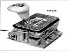
Potentiometer for recognition of selector lever position
