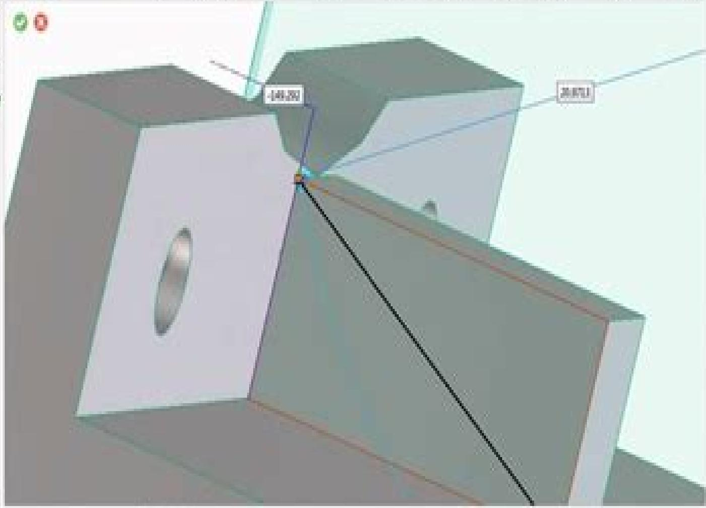
Specify the second point of the line or enter the line length in the given direction.
