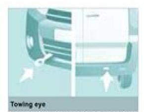
At the front, unclip the cover by pressing it at the bottom.
