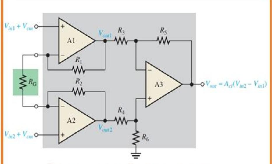
The basic instrumentation amplifier with an external gain-setting resistor RG. Differential and common-mode signals are indicated
