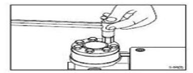
(32) Place the dust seal ring in the housing.
