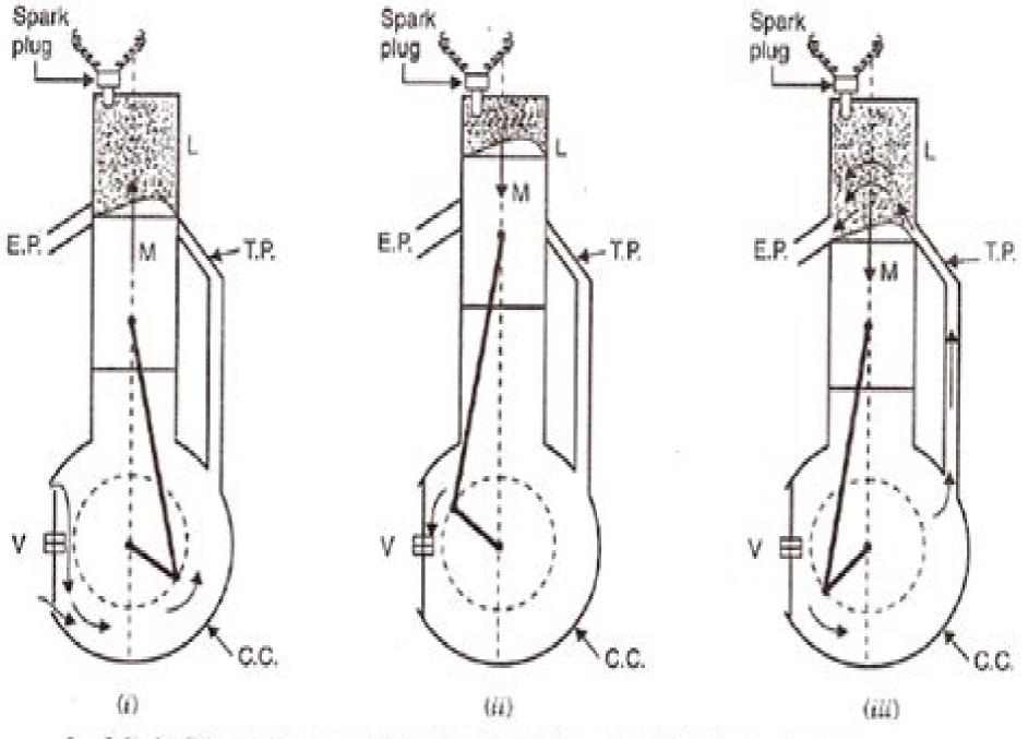
L = Cylinder E.P. = Exhaust port T.P. = Transfer port V = valve, C.C = Crank chamber
