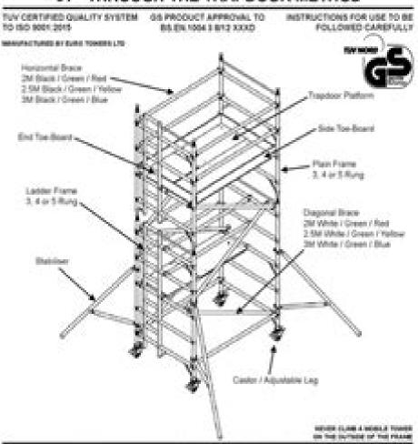
MAX SAFE WORKING LOAD FOR TOWER 750KG MAX SAFE WORKING LOAD PER PLATFORM 250KG
