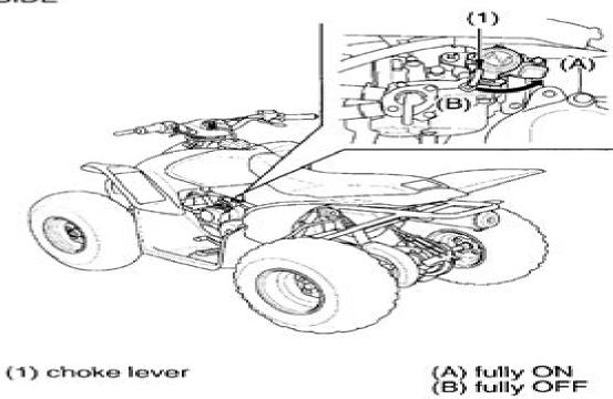
The choke lever may be used when starting the engine. See page 56.
