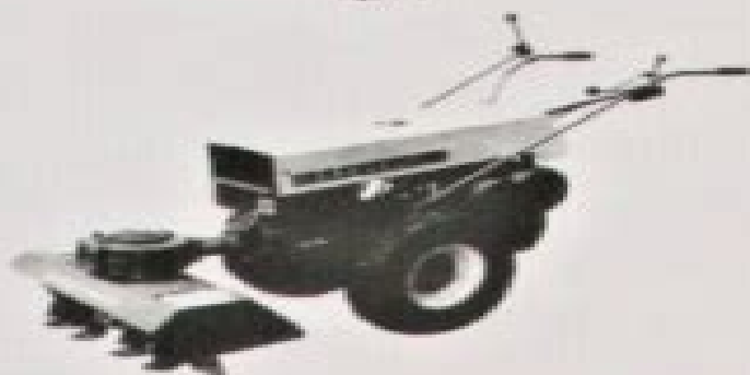
1557BE1 Rotary Cultivator mounted on Commercial 15A Cummins Engine. When Used: 1.5 HP Commercial, Commercial 15A and 1.5 Commercial Tractor. Additional Equipment Required: 1557BE1 Rotary Flow or 1557BE1 Flow-Cultivator Drive. Additional Equipment Recommended: None.
