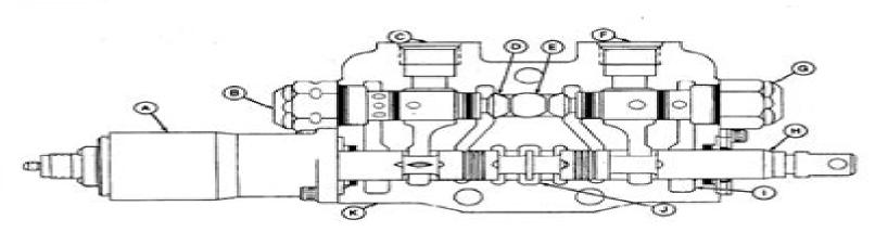
A—Solenoid B—Relief Valve with Anti-Cavitation C-To Head End of Cylinder D-Lift Check Poppet (2 used) E-Power Passage
