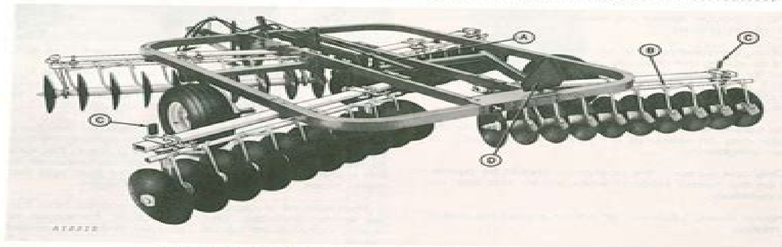
C—Reflector D—Slow Moving Vehicle Emblem
