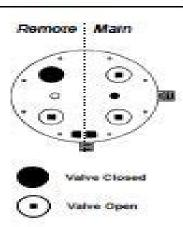
Main Tank is in Service and Remote Tank is in Backwash.
