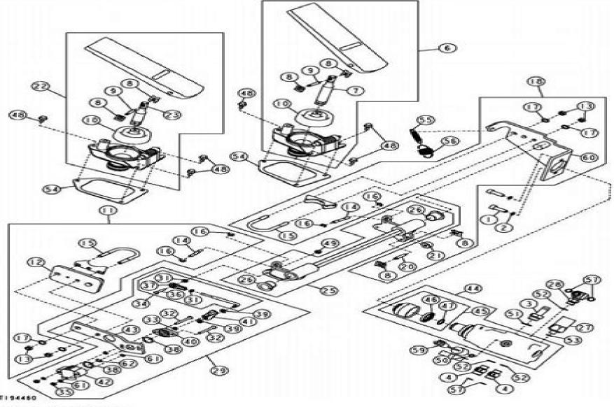
Brake Pedal and Linkage
