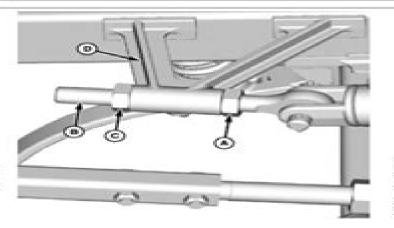
A—Front Jam Nut B—Eyebolt C-Rear Jam Nut D-Bracket
