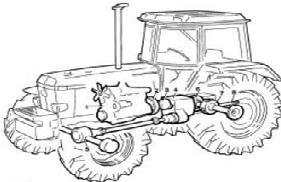
Fig. 1 – Power Train Components
