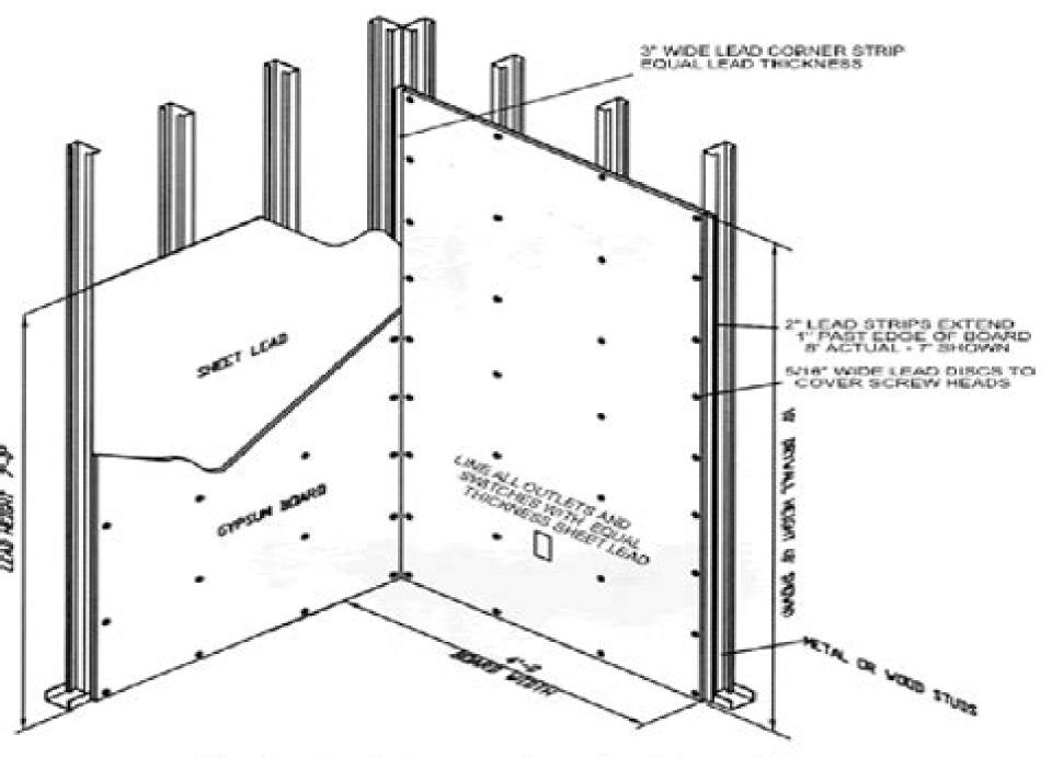
Fig. 1. A typical geneum board wall accombly.
