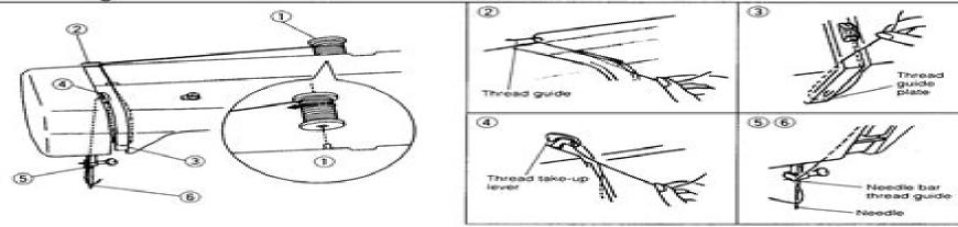
Raise the Thread Take-up lever to its highest position by turning the Hand Wheel toward you. Raise the Presser foot.
