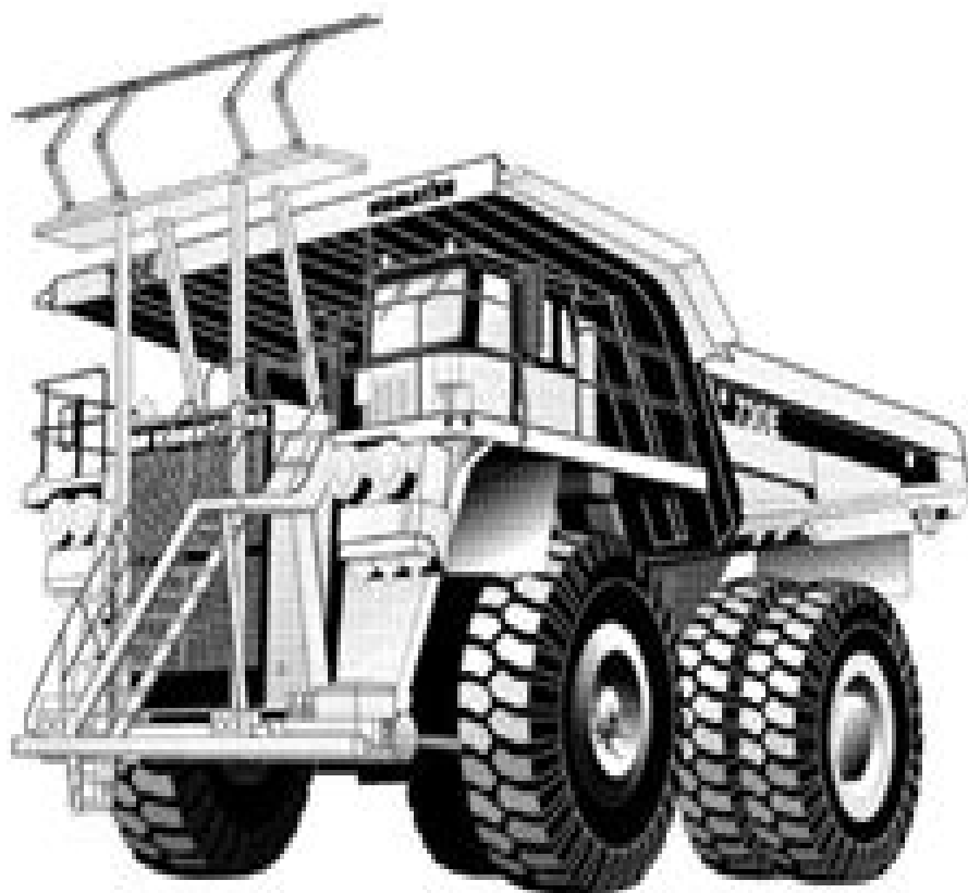
KOMATSU MODEL 730E DUMP TRUCK WITH TROLLEY ASSIST
