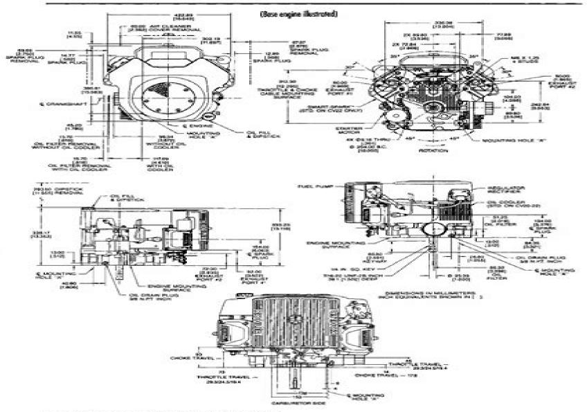
Figure 1-4. Typical Engine Dimensions CV17-22.
