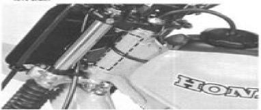
The carburetor identification number is on the carburetor body right side.
