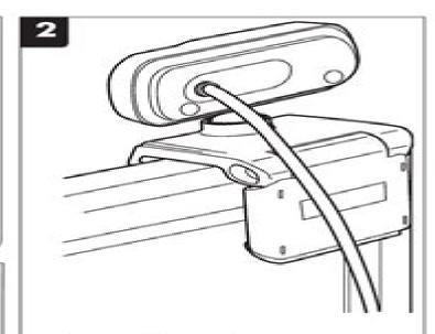
Mount the webcam on your monitor. Unfold the foot and rotate the ball joint as desired.
