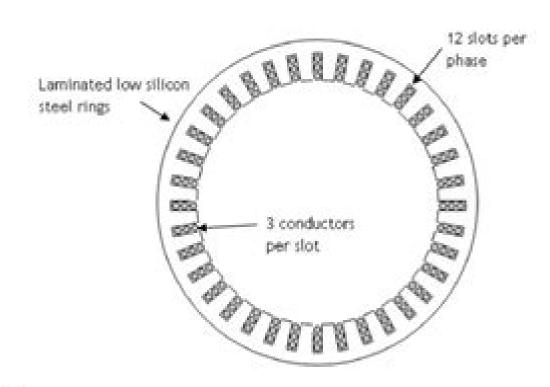
Example of 36 slot stator
