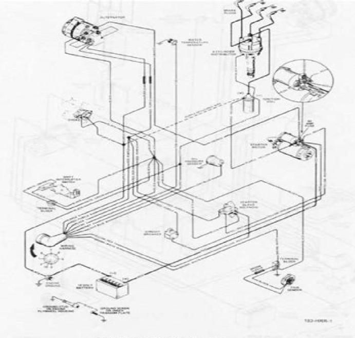
MCM 120R/140R Engine Wiring Diagram with 90 Amp Fuse at Starter Motor (Orange Wire) Mando Alternator (Battery Meter Circuit)
