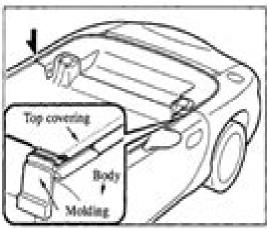
Insert the top covering's rear edge into the groove in the body molding.
