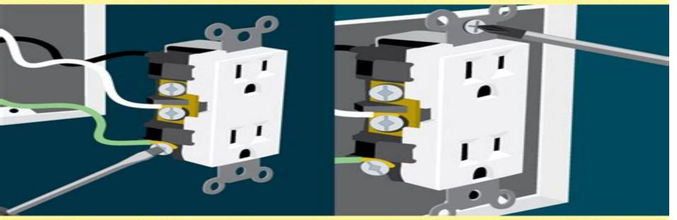
Using your flathead screwdriver tightly screw the wires into the new outlet. Screw the outlet back into the box with the two Phillips screws.
