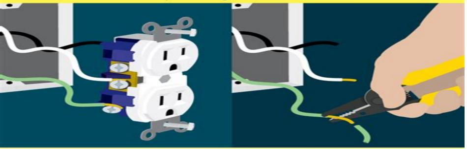
After removing the screws which hold the outlet in place, gently pull it out of the box.
