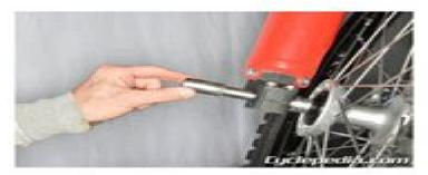
Support the wheel and remove the axle bolt.
