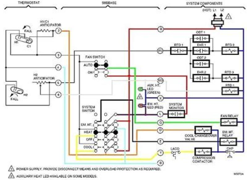
Fig. 6. Internal schematic and typical wiring diagram for Y594R1243 (T874R1152/Q674L1207).
