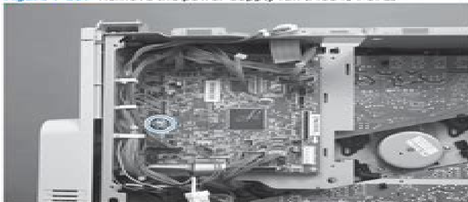
Figure 1-297 Remove the power-supply fan (M651; 1 of 2)
