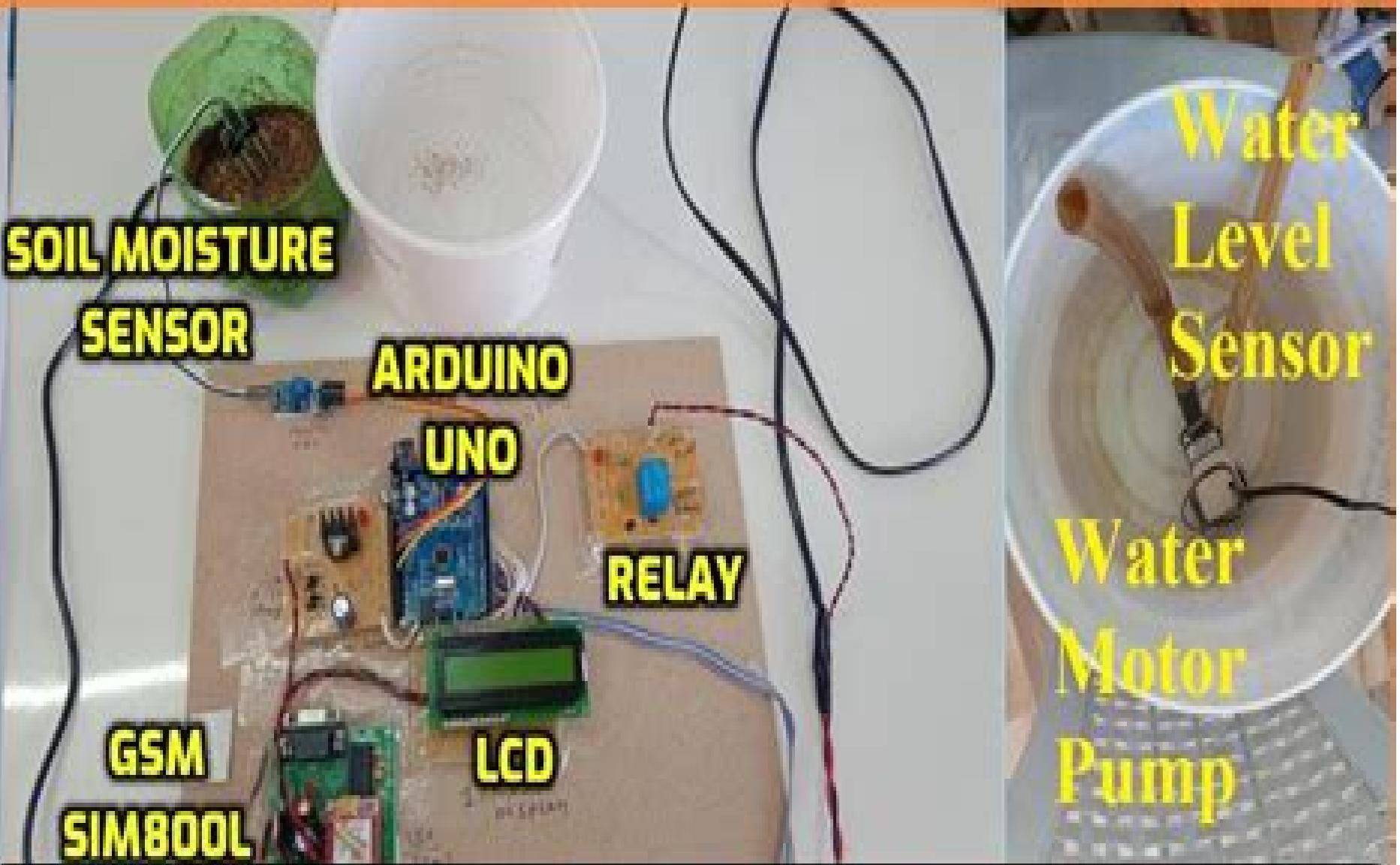
**GSM Based Motor Controller in Irrigation by Using Sensor's
