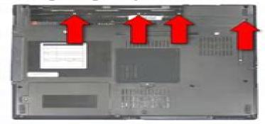
Remove 3 screws from inside the Battery Bay. Remove one screw from the rear of the Lower Cover.
