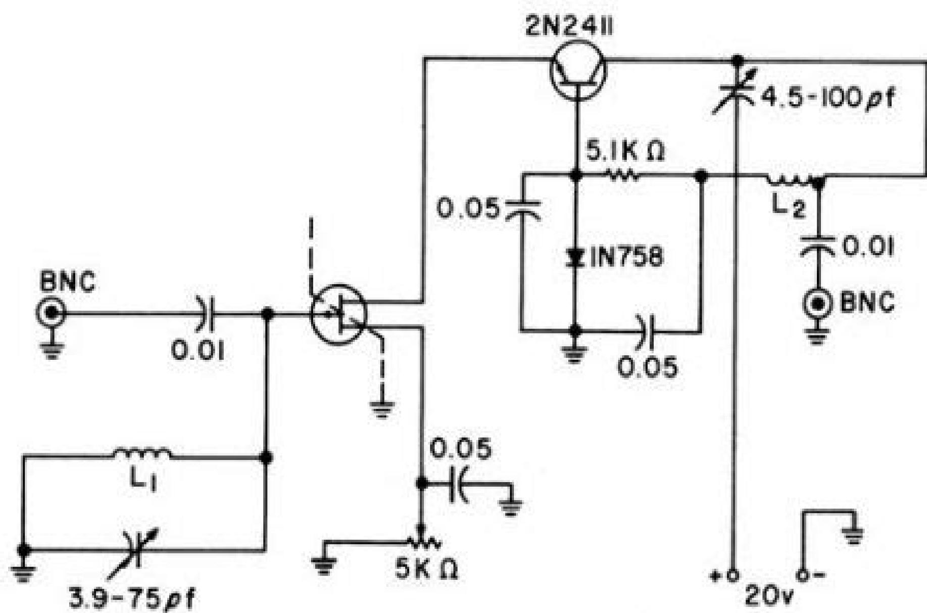
$L_1$ ,  $L_2$  18 turns B&W 3004 Minductor;  $L_2$  tapped  $1\frac{3}{4}$  turns from ground.
