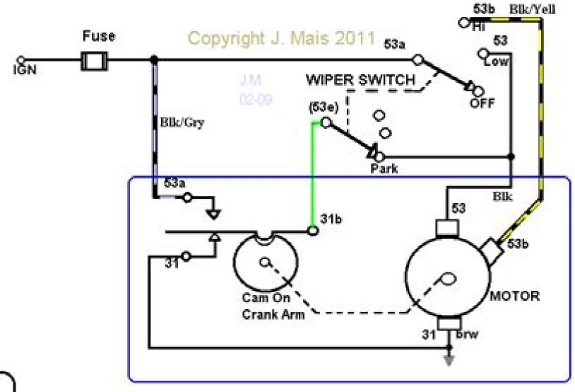
Motor Internal Wiring
