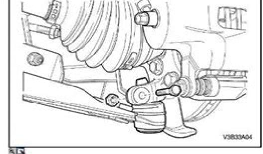
4. Remove the lower ball joint nut and bolt.
