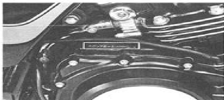
The engine serial number is stamped on top of the right crankcase.
