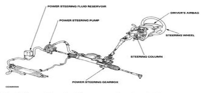
Fig. 2: Power Steering Component Location Index Courtesy of AMERICAN HONDA MOTOR CO., INC.
