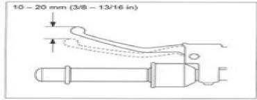
The adjuster may be damaged if it is positioned too far out, leaving minimal thread engagement.
