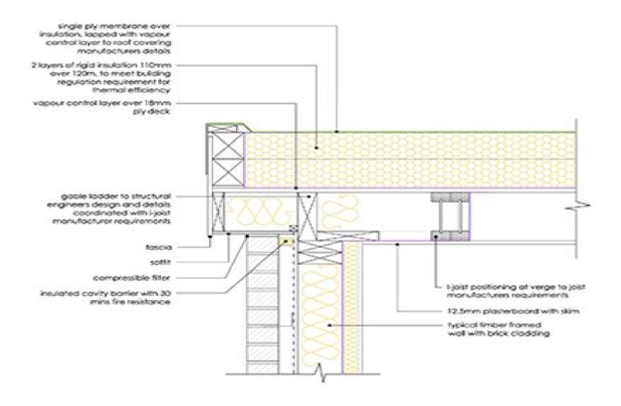
7 I-joist flat roof to timber frame wall - verge detail
