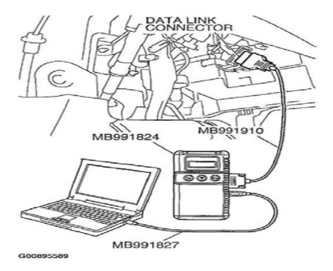
Fig. 4: Connecting Scan Tool MB991958 To Data Link Connector Courtesy of MITSUBISHI MOTOR SALES OF AMERICA.
