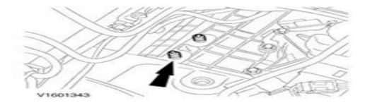
19. Remove the four upper bellhousing bolts.
