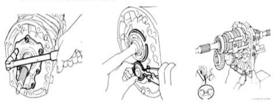
Remove the front bearing retainer & snap rings, a separate intermediate plate from the transmission case, and mount the intermediate plate in a vice.
