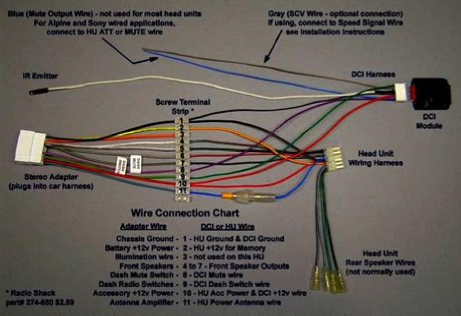
Note: This drawing shows an IR OCI, but the wiring is similar for all types of DCI's. Different HU brands may have different wire colors on the HU Wire Harmess, so check your head unit manual before wiring.
