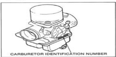
The carburetor identification number is on the carburetor body right side.
