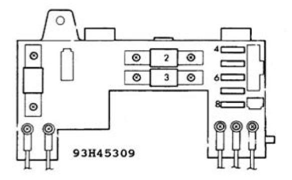
Fig. 2: Underbood Fuse Panel Identification (1988-91) Courtesy of AMERICAN HONDA MOTOR CO., INC.
