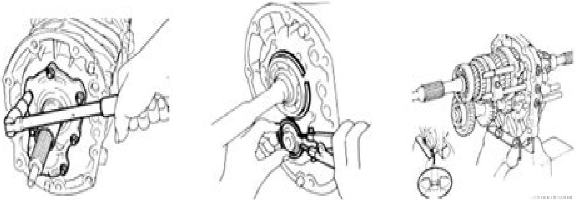
3. Remove the front bearing retainer & snap rings, a separate intermediate plate from the transmission case, and mount the intermediate plate in a vice.
