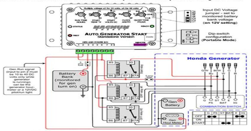
Relays used are SPDT 30 Amp, 12 VDC coil relays [shown in the non-energized (N.C.) position]
