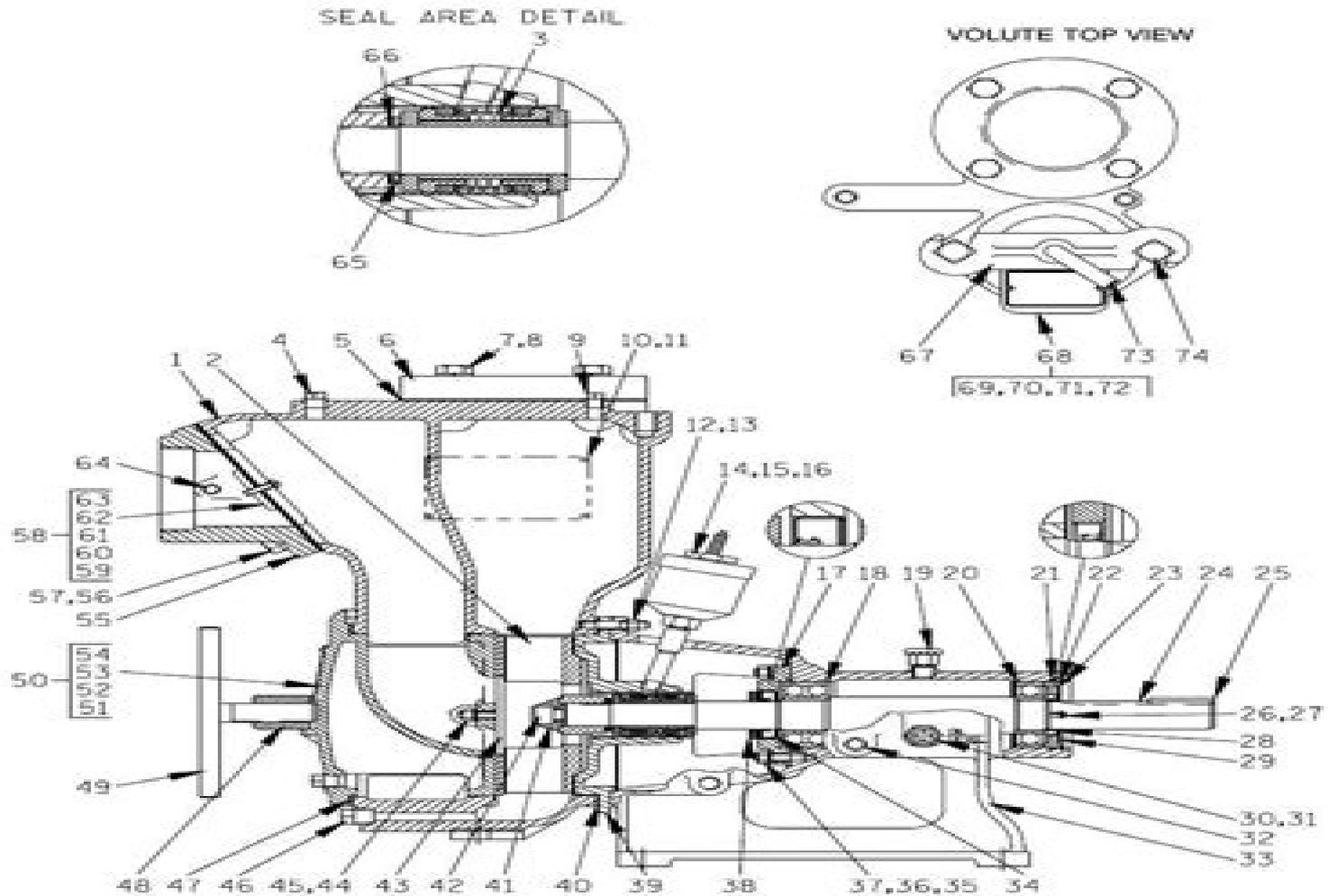
Figure E-1. Pump Model 14A2-B
